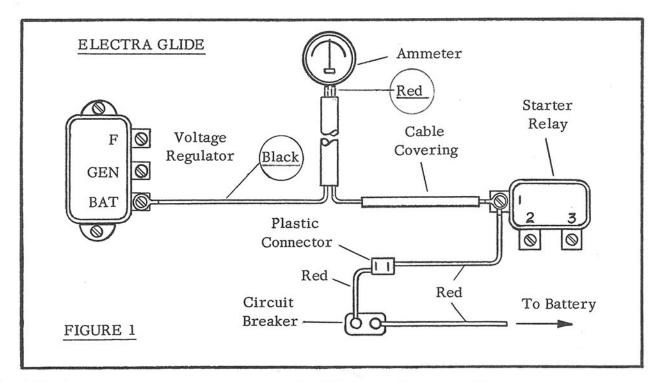
Lead black ammeter wire up to regulator "BAT" terminal and cut off excess. Crimp and solder one ring terminal from kit onto wire and attach wire to "BAT" terminal, along with remaining red wire from terminal box. Reinstall regulator.
