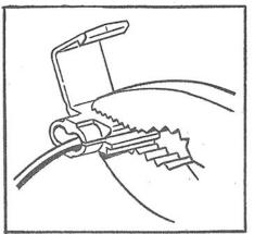
2. Use pliers to squeeze down metal clip. Clip shears through insulation and grips wires tightly.
