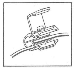
1. Place wire ends into connector so that ends are past middle notch.
