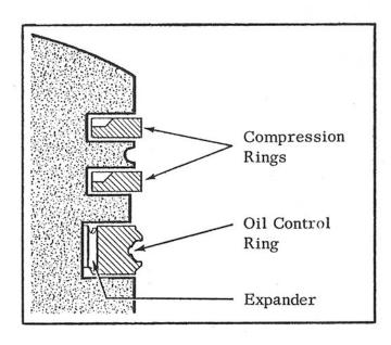
A two-piece oil control ring has been in use on the Sportster and Electra-Glide engine since the start of the 1966 model season.
