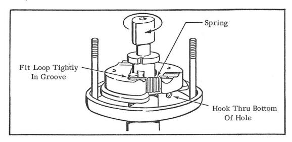
On 1967 and later models, also see that bent end of each flyweight spring is hooked through bottom of hole and see that upper looped end of each spring grips retaining groove in pin tightly.
